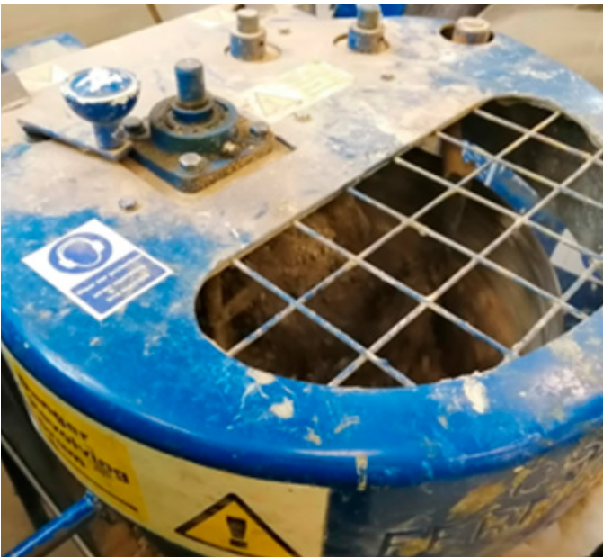
Figure 11: Pan Mixer of 0.05 m3 Capacity Employed for Concrete Mixing.
