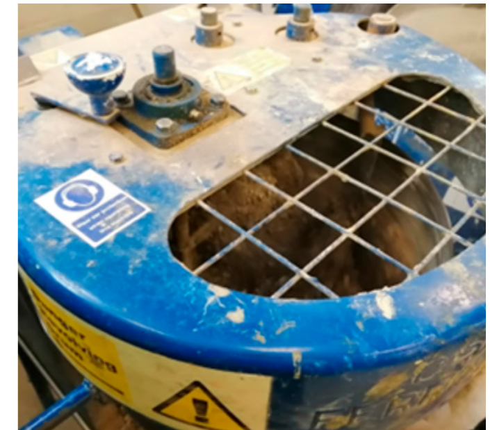
Figure 11: Pan Mixer of 0.05 m3 Capacity Employed for Concrete Mixing.
