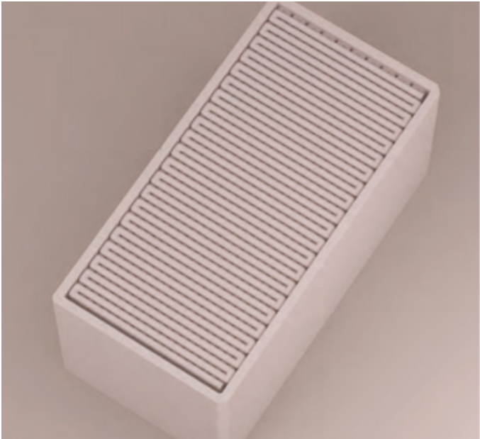
(b) Simulation of full deposition Simulation of full deposition to create a 3D printed block using recycled aggregates.
